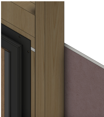
Insert Fyreline Gib Into Frame GIB Groove All Sides
