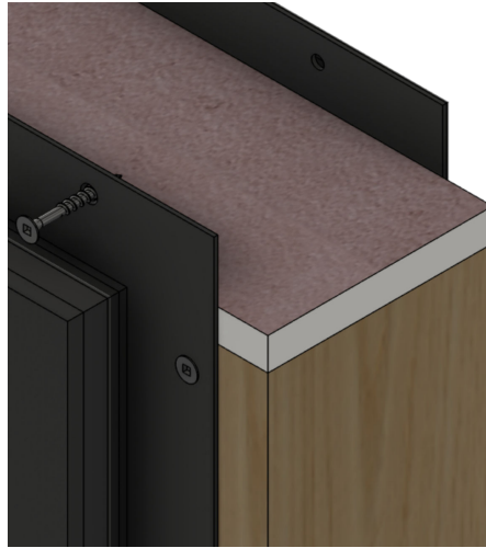
Add 13mm Fyreline GIB On Top of Frame
