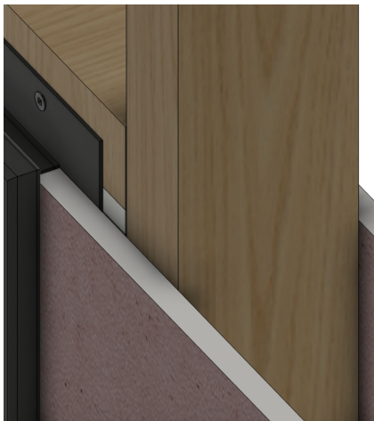
Align Fyreline Gib With Top GIB Groove
